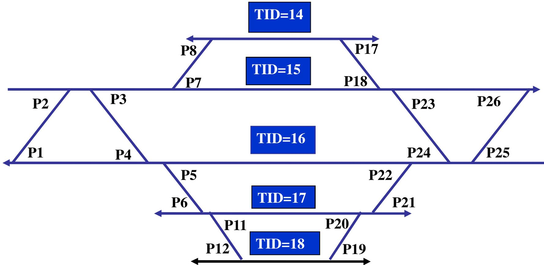
Database of TID Plans of Stations, GPS shadow zones, Level Crossings and Repeaters on ACD Routes are stored in memory of 'Loco' & 'Guard' ACDs
